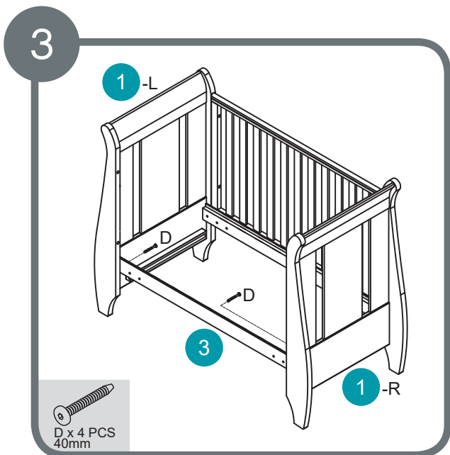
Assemble front mattress support bar using 4 x D bolts
